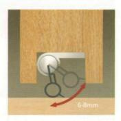
Standard design suits thresholds gaps between 6 - 8mm. Designs for gaps up to 12mm available on request.
